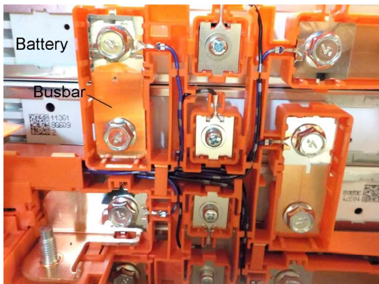
Inside of a Li-ion HV battery
