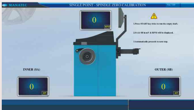
Step by step self calibration procedure guides the user to perform calibration easily & quickly.
