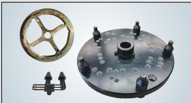
Universal flange kit is designed to eliminate wheel fixing errors and achieve better results
